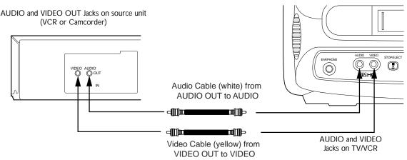
Make the connections shown above, using audio and video cables. (Make sure the source unit is connected to a power source.)
